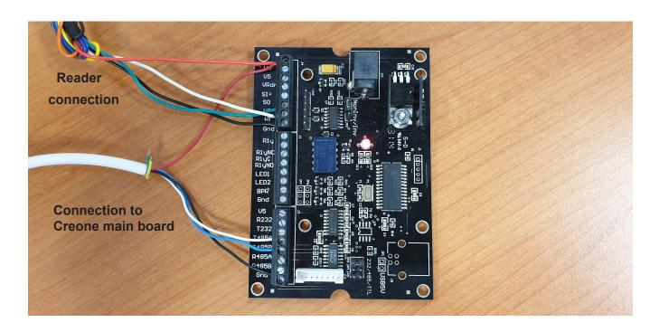
The remaining wires in the picture above are for the RS485 signal attached to the Creone Keybox main control board shown in order from bottom to top of the terminal block: (Red Voltage +, Black Gnd, Blue 485B, White 485A)
